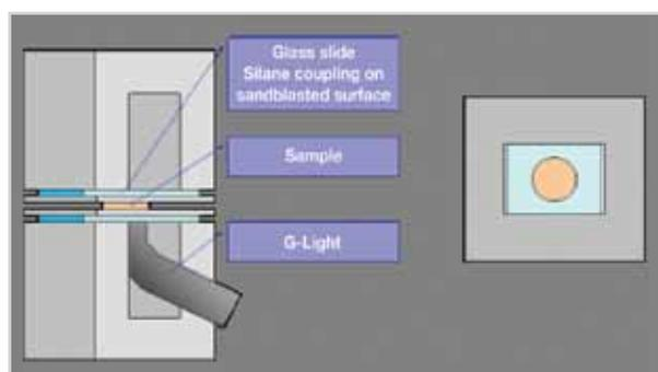
The sample was light-cured for 40 seconds from the underside using a G-Light 11mm fiber rod, then light-cured for 20 seconds from above. The setting shrinkage stress was measured for 20 minutes and the highest figure reached was recorded as the shrinkage stress.
