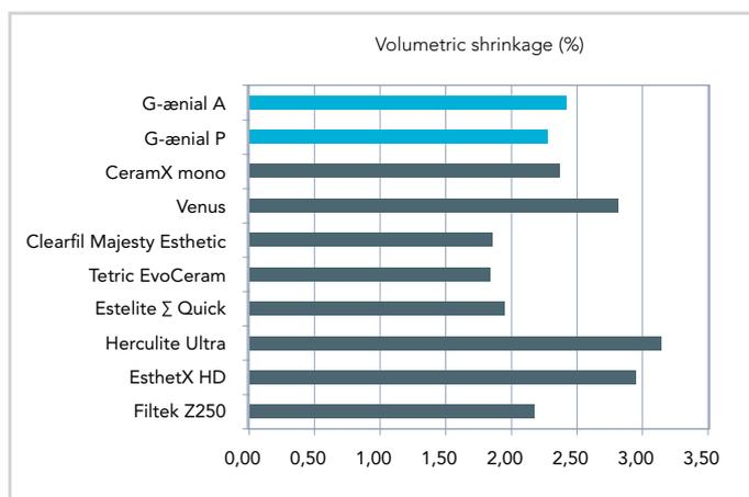
The volumetric shrinkage was measured following ISO Draft Date: 2007-07-10 (Dentistry - Polymerization shrinkage of filling materials) specifications.
