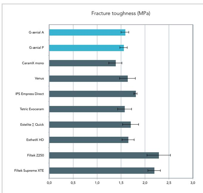
Test method is based on ASTM E-399, Fracture toughness test
