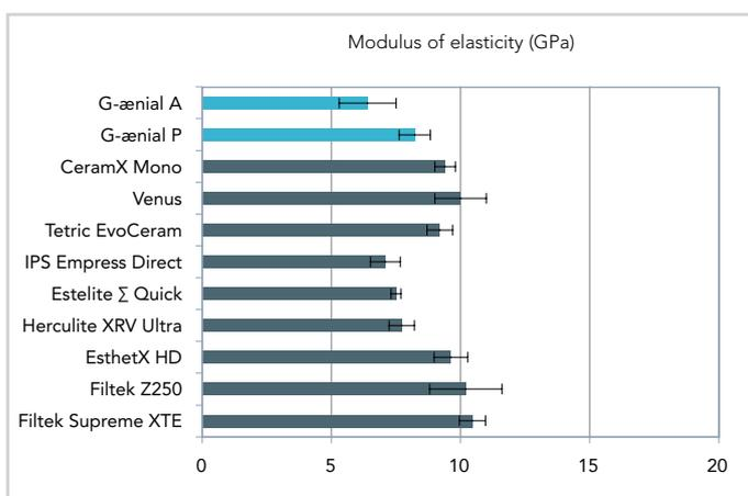
The modulus of elasticity of G-ænial was determined according to the ISO 4049:2000 specifications.
